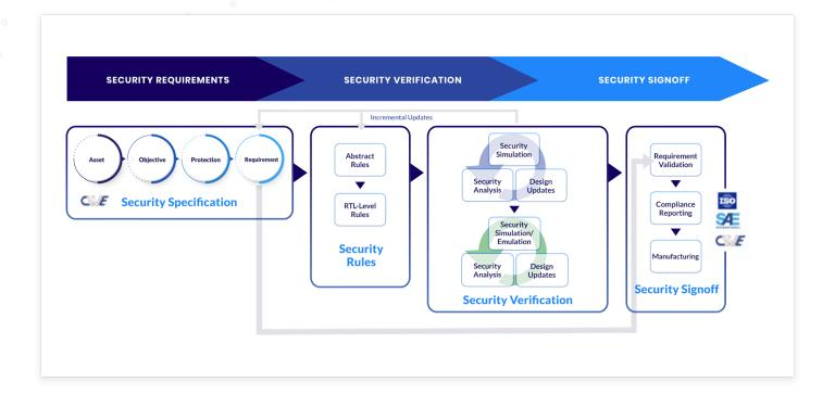
The Radix rules, combined with the simulation and emulation tests, establish the security verification plan.
